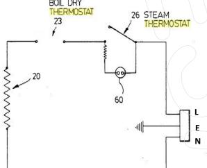
The schematic diagram on the left is of the electrical circuit of a standard kettle and it shows the operating circuit the appliance mains lead connects to. The following is only considering the 'Insulation Resistance' test of the PAT test procedure in order to illustrate the need for knowledge and practical experience of product when testing appliances.
