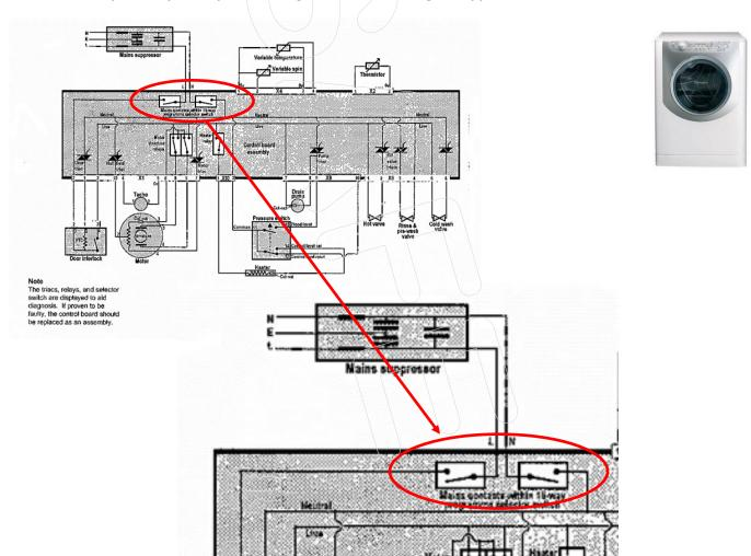
Normally 'Open' relay switches are found on many products - washing machines, washer dryers, dishwashers, microwave ovens etc. in-depth appliance technical and practical knowledge is therefore required when testing such products.
